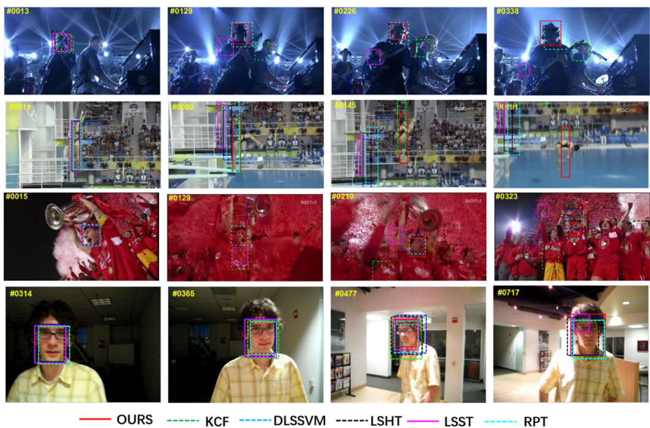
Fig. 1 The proposed tracker performs more favorable in dealing with “Shaking” (first row, with 5 challenges: IV, SV, IPR, OPR, BC), “Diving”(second row, with 3 challenges: SV, DEF, IPR), “Shocker”(third row, with 8 challenges:IV, SV, OCC, MB, FM, IPR, OPR, BC) and David (fourth row, with 7 challenges: IV, SV, OCC, DEF, MB, IPR, OPR)
